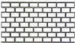
Running Bond Brick Size - 4" x 7 3/4" Joints - 1/2"
